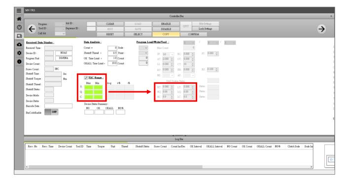
LOAD: To load the parameter settings from the KL-MCTDS5 controller.
