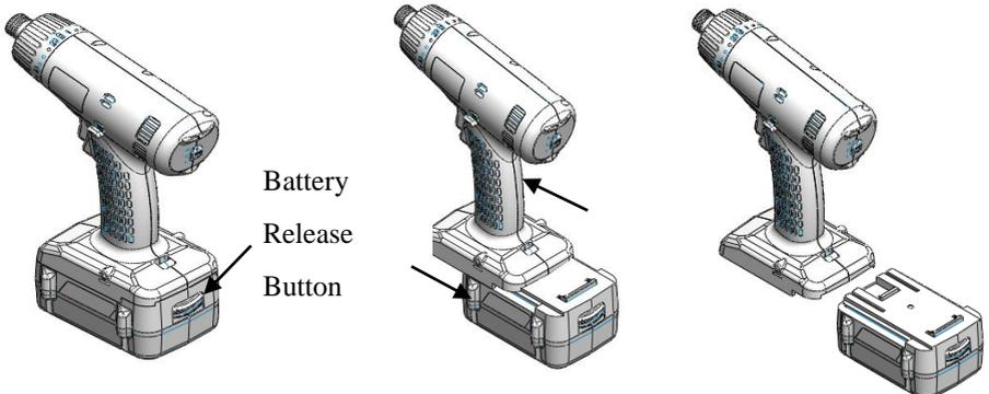
(1) Press the release button and take it out of the device.
