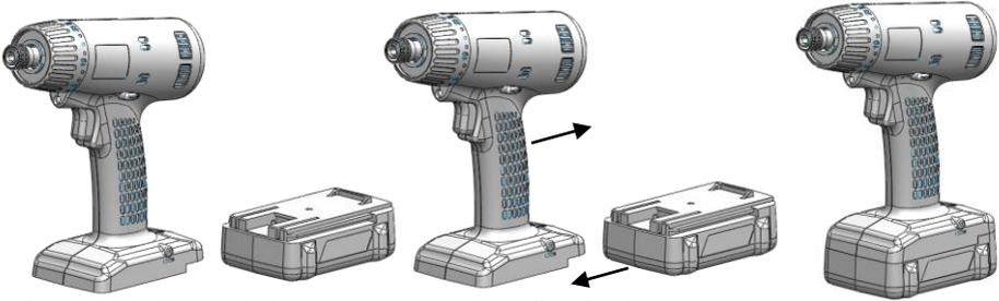
(1) Insert the rechargeable battery into the device follow by the arrow as showing.
