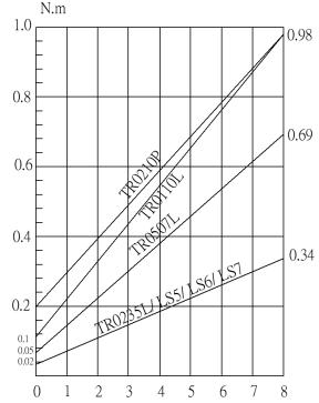
7. The torque checker measures the torque of screwdriver. The clamping torque of screw itself is different from the clamped conditions. Understand the correlation between clamping torque values and the torque checker values perform the torque control properly.
